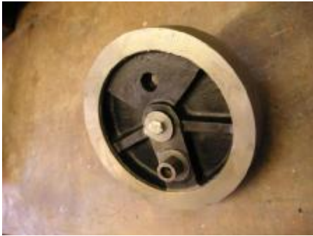
Tyre fitted before final machining of rim.
