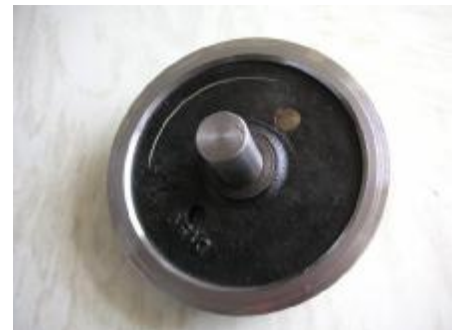
Rear of wheel. Note mandrel for holding it while machining.
