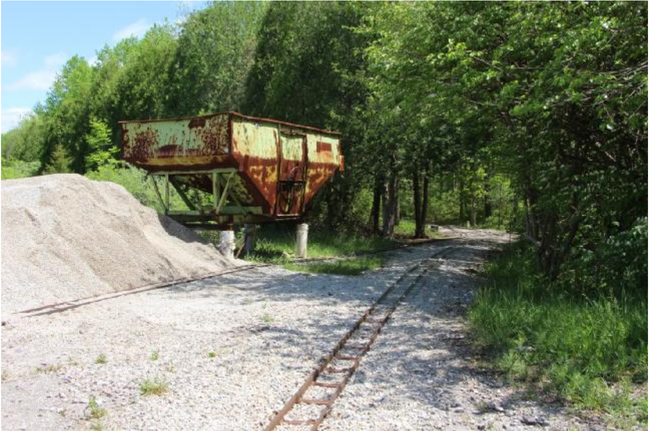
A hopper converted to hold ballast for MoW
